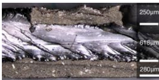
Fig. 5. Cross-section of the microstrip line.
