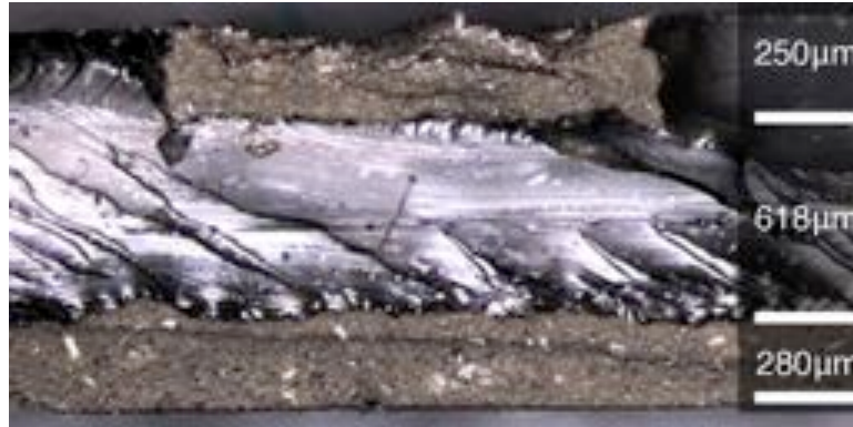
Figure 63. Cross-section of stretchable microstrip line after testing [196].
