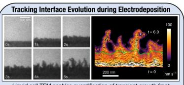
Liquid cell TEM enables quantification of transient growth front dynamics during electrodeposition of copper. The growth undergoes a transition at ~ 3s after which the roughness of the growth front increases more rapidly. (Schneider et al., 2017).
