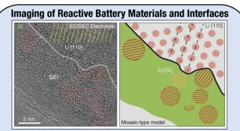
Cryogenic cooling in TEM allows reactive materials such as lithium metal to be imaged at atomic resolution. The structure of the solidelectrolyte interface (SEI) layer that forms on the surface of the Li electrode during battery cycling is resolved (Li et al., 2017).
